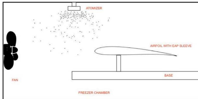
Figure: Sketch of experimental setup
