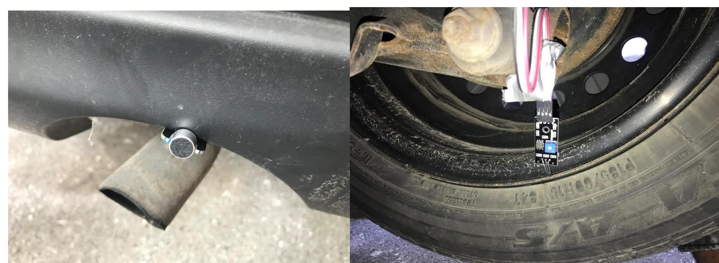
Figure 2: Testing Done on Personal Vehicle Using Sound Sensor (Left) and Hall Effect Sensor (Right)
