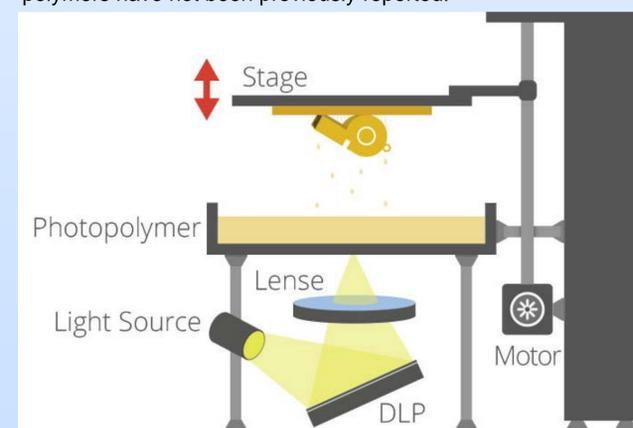
3D printing by stereolithography with bottom-up projection
