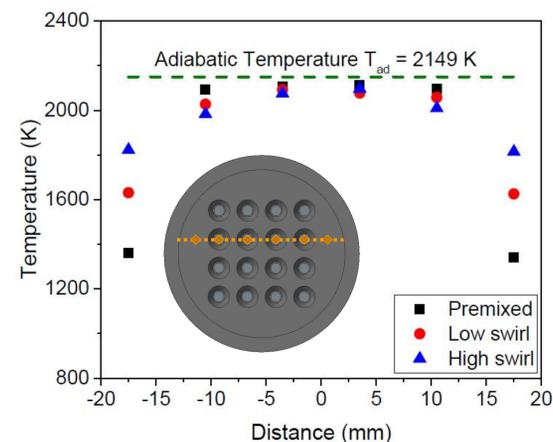
Figure 7: Spatial temperature distribution at 25mm above the burner array surface under various swirl stabilized configurations ( $\phi = 0.95$  and total flow rate of 10k scc/min)
