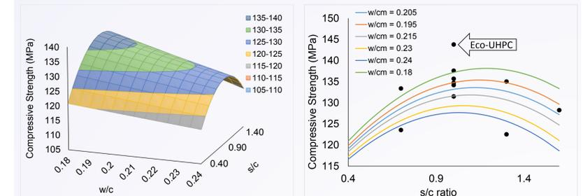
Figures 6 and 7: Relationship between compressive strength and design variables
