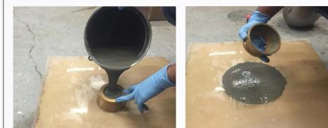
Figure 3: Mini-Slump Test:
