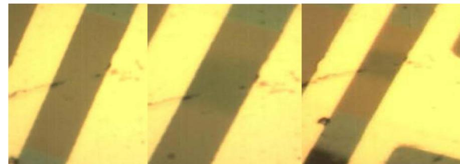
Figure 8: Insulating 100x (left)/ Conducting domain 100x (center)/ Conducting domain 50x (right)
