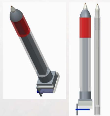
Pictured to the left is the CAD model of the prototype cyber-empathic pen. There are 2 force sensors in the pen located underneath the grip. There is another force sensor at the back of the pen measuring the force being used to press down. There will also be an accelerometer attached to the back of the pen to track user movements when writing.
