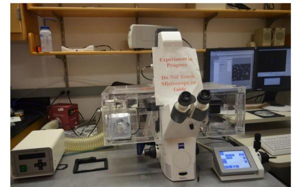
Figure 5. The Zeiss Axio Imager Z1.
