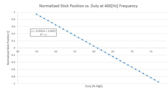
Figure 8: Normalized stick position vs. Duty
