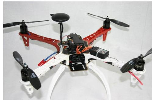
Figure 2: Base DJI F450 Quadcopter Kit with GPS Navigation
