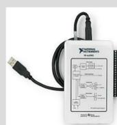
The myDAQ is a data acquisition device fully compatible with the National Instruments products MultiSim and LabVIEW that we are using. This device provides the analog to digital conversion for data acquisition and interface with a PC. It is USB compatible with the equipment we are using for design verification and also has the capability to be used as an ammeter and voltmeter.
