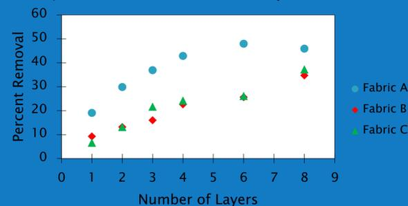
Figure 4: Removal of Low Turbidity
