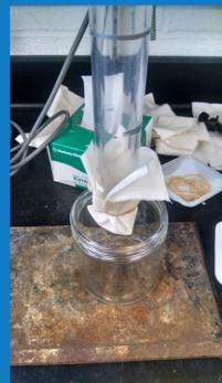
Figure 2: General Setup of Filter
