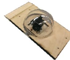
Figure 5: Camera Fairing and Fuselage Mount
