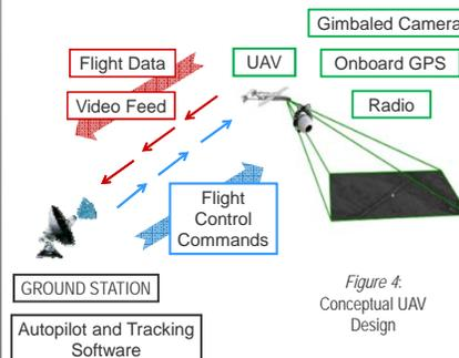
Figure 4: Conceptual UAV Design
