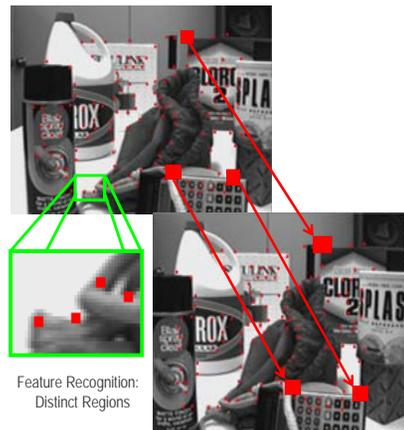
Figure 3: Corner Detection and Tracking
