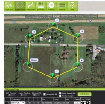
Figure 6: Mission Planner Example Flight Plan [1]
