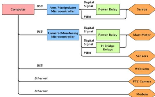
Figure 1 – Control and Communications System
