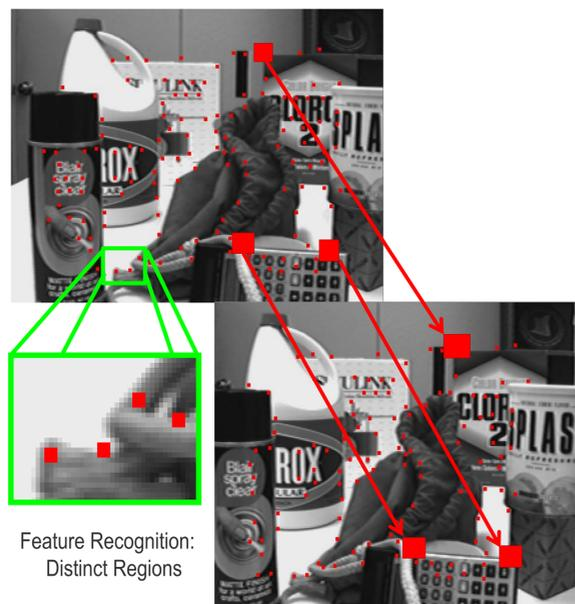
Figure 3: Corner Detection and Tracking
