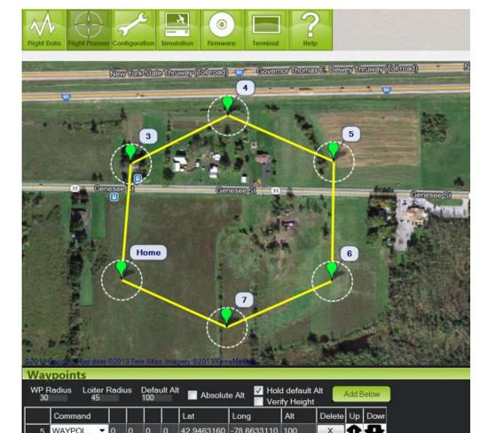
Figure 10: Mission Planner Example Flight Plan [4]
