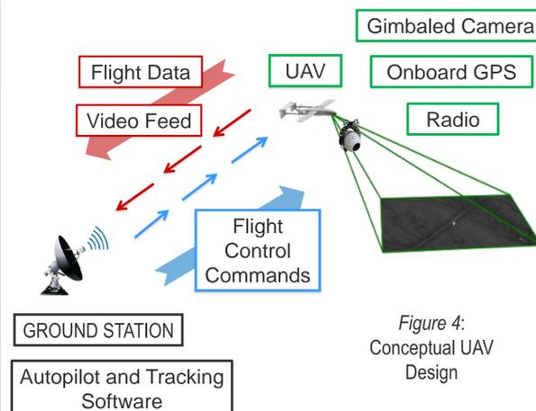
Figure 4: Conceptual UAV Design
