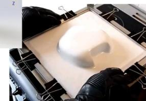
Figure 6: Thermoforming Process [1]
