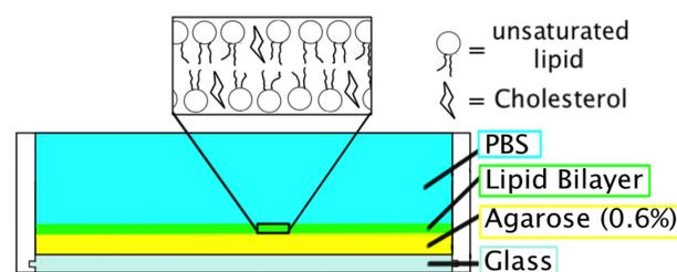
Figure 1. Schematic of agarose supported lipid bilayer: Agarose and lipid mixture are spin coated on top of clean glass. The sample is hydrated with 3X PBS to form lipid bilayer.
