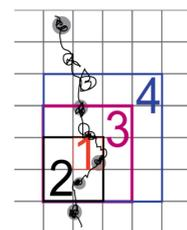
Figure 2. By altering binning of the camera pixel during analysis, different area for FCS analysis can be produced. Information about possible domain smaller than the pixel size (grey dots) can be extrapolated from the series of FCS data generated.
