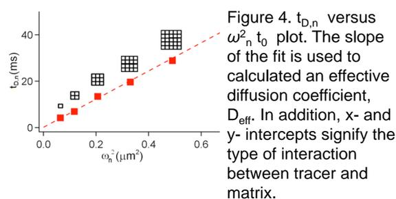
Figure 4.  $t_{D,n}$  versus  $\omega_n^2$  plot. The slope of the fit is used to calculate an effective diffusion coefficient,  $D_{eff}$ . In addition, x- and y- intercepts signify the type of interaction between tracer and matrix.
