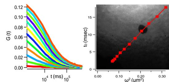
Figure 6. BimFCS on Liss Rhodamine-PE marker within the agarose supported DOPC bilayer. Diffusion is significantly faster than in the solid supported system. ( $D = 6.2 \pm 1.2 \mu\text{m}^2/\text{sec}$ )
