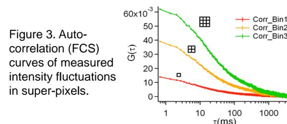
Figure 3. Auto-correlation (FCS) curves of measured intensity fluctuations in super-pixels.
