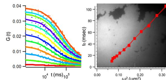
Figure 5. Liss Rhodamine-PE diffusion in a solid supported DOPC bilayer measured by bimFCS. ( $D = 1.2 \pm 0.2 \mu\text{m}^2/\text{sec}$ )
