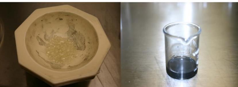
Fig. 1. The Pliogum has been soaked in toluene for a period of time in the mortar.
