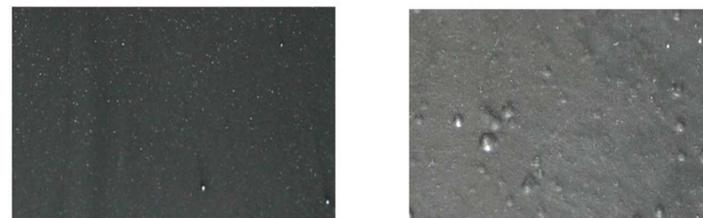
Fig. 7. A close up of both samples shows the composite on the right with more air bubbles and pieces of undissolved rubber.
