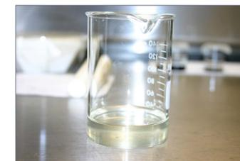
Fig. 8. 150 mL beaker with 1.5 g of Plioflex 1502 in 40 mL of toluene.
