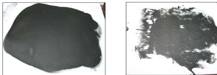
Fig. 6. On the left is a composite of Plioflex 1502 and graphene. On the right is Pliogum 1027 with graphene.
