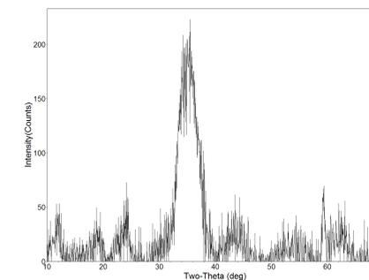
Figure 6: Experimental XRD pattern for  $MgFe_2O_4$ .
