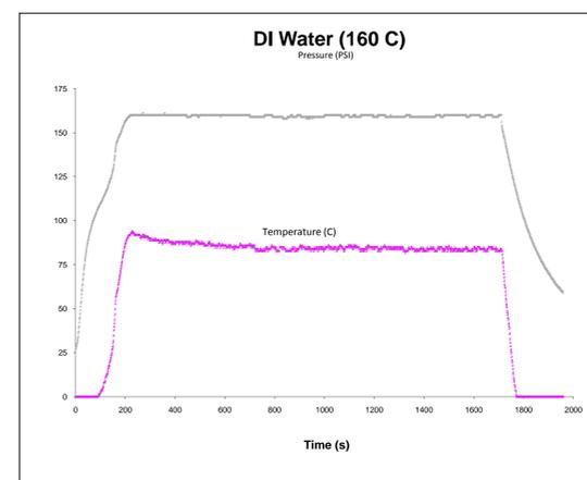
Figure 4: Sample water test showing temperature/pressure relationship for water.
