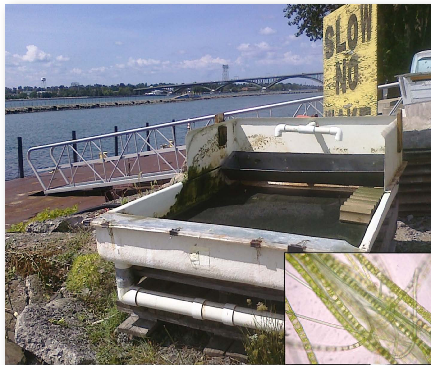
Figure 1: An ATS set up at the Great Lakes Center location on the Black Rock Canal; lower right: An image of Chladophora algae under a microscope.
