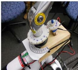
Figure II. Steering position sensor
