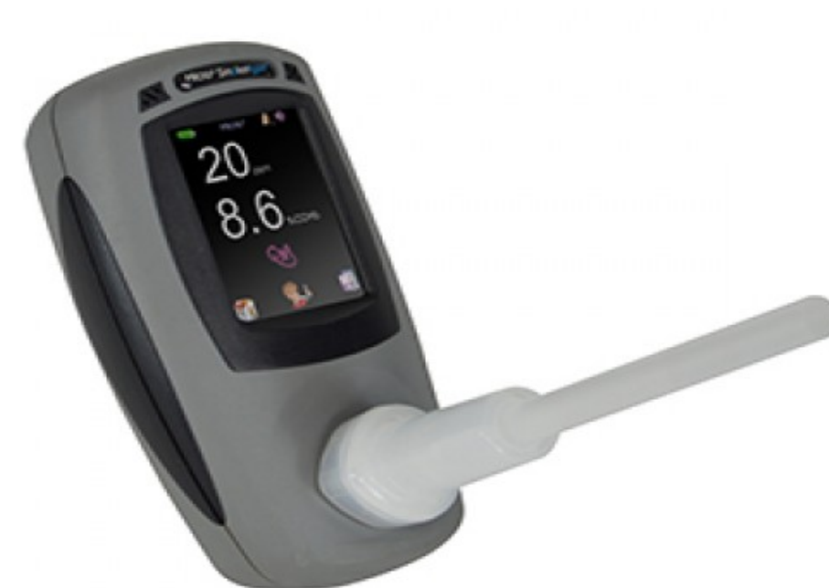
Fig. 3: Breath Carbon Monoxide (CO) test gives the concentration of CO in mothers as well as fetal hemoglobin CO levels.
