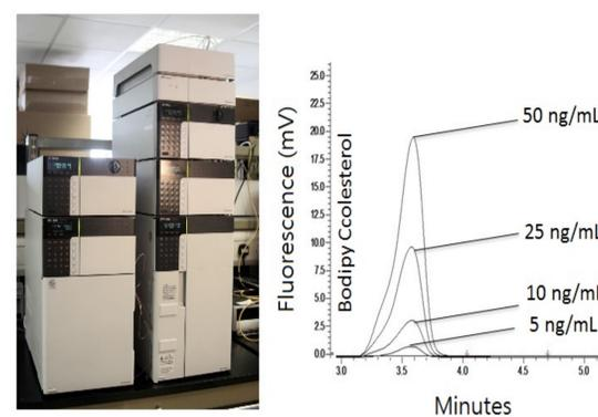
Figure 4: HPLC – Fluorescence system (left) and chromatogram (right)
