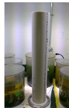
Figure 1. Tube used to determine rhizoid length. Tube was placed directly under lamp to ensure normal exposure. The bottom is removable.
