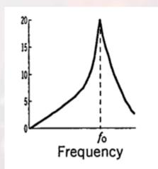
The graph above displays output voltage vs frequency of an induction loop, where  $f_0$  is the resonance frequency. (Macintyre,98)
