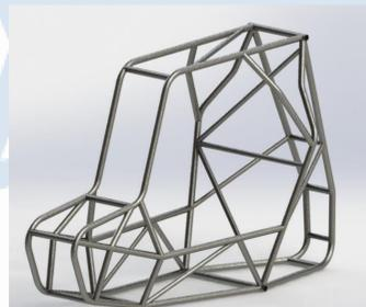
The second concept was radically different due to the in-swept Rear Roll Hoop members. This design change was projected to greatly reduce firewall drag forces.
