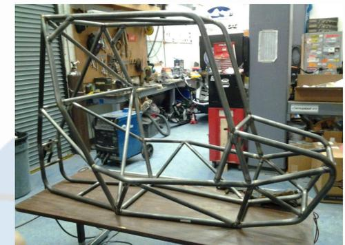
The above picture shows the space frame after assembly and welding. The assembly process and sub-assembly fitment was as anticipated from the SolidWorks analysis.
