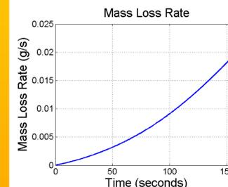
Figure 8: The mass loss rate of the sample is plotted as a function of time. The data is acquired through instantaneous mass measurement of the PMMA sample.
