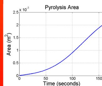
Figure 7: The pyrolysis area is plotted as a function of time. The data is acquired through image processing of the images of the pyrolysis region.
