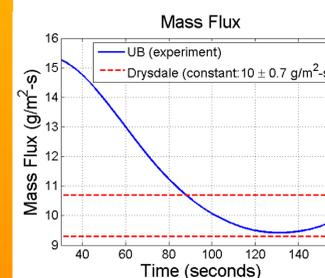
Figure 9: The mass flux is plotted as a function of time. Obtained by dividing the mass loss rate by the pyrolysis area, both of which were measured simultaneously.
