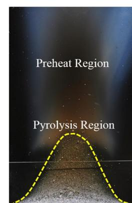
Figure 2 - (left) A digital photograph taken at UB of the pyrolysis region where the moving pyrolysis front is highlighted in yellow. The preheat region is labeled as well.
