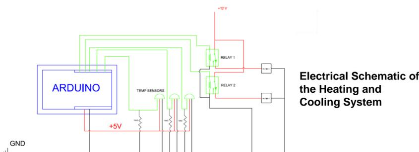
Electrical Schematic of the Heating and Cooling System
