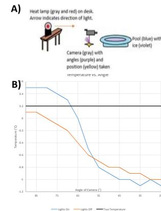
Figure 6: (A) Lab testing setup and (B) deviation in temperature due to angle of incidence.
