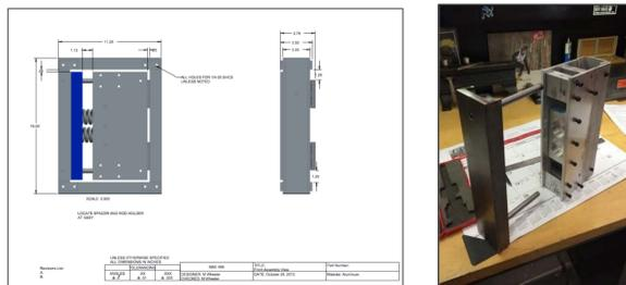
Figure 1 and 2: Detail Drawing and partially manufactured assembly
