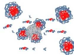
**Figure 4.** PEO promotes a homogenous surface coating on the particles—containing both P105 micelles (smaller than typical) and PEO chains.
