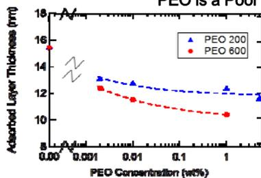
**Figure 3.** Adsorbed layer thickness observed for Pluronic P105-stabilized silica dispersions in the presence of (▲) PEO 200 or (●) PEO 600 plotted versus the logarithm of added PEO homopolymer concentration (wt%).
