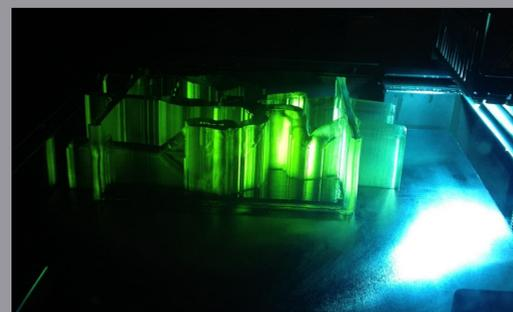
The 3D printer uses UV light to cure each layer of material.
