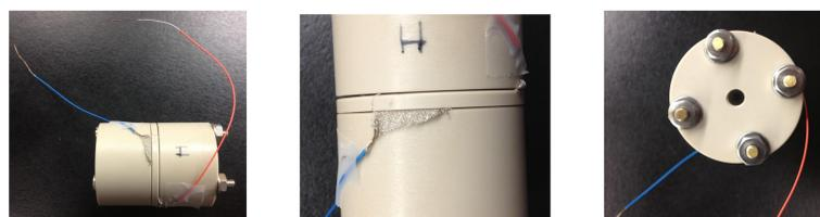
Full view of the EK micropump along with a close up of the wires secured to the mesh platinum electrode and a view of how the pump components are connected.
