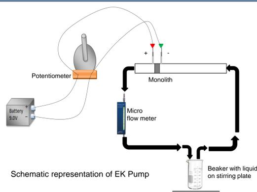
The voltage applied to the EK pump is supplied by 9V batteries connected in series. The potentiometer allows control of the voltage being applied across the monolith using platinum electrodes. The monolith is encapsulated in a plastic tube. The generated flow is measured via a microflow meter.
