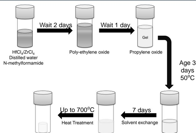
$\text{HfO}_2$  and  $\text{ZrO}_2$  monolithic structures were synthesized by sol gel processing.
