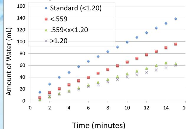
Figure 2: Hydraulic Conductivity
