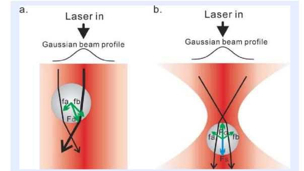
The optical trap is a function of the particle-like properties of light. The momentum of light exerts many forces on the bead. Propagation of light through the particle also causes various directional forces on the particle.
