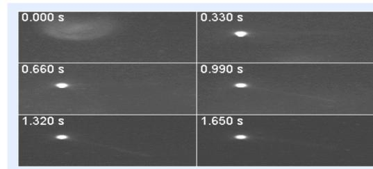
This is a montage of images that display use of the optical trap to capture a bead-bound λ-DNA molecule. The bead is the fluorescent white circle. Behind it is a faint gray line.
