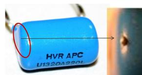
Figure 6. A crack in the resistor (a).
