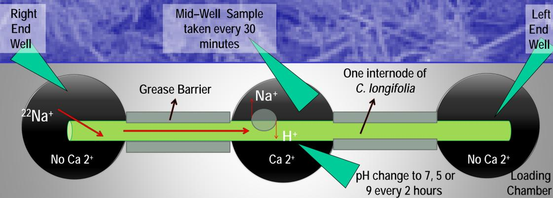
Fig. 1: Schematic diagram of method of efflux measurement
