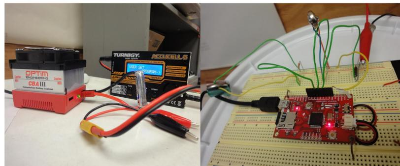
Fig. 1. The test setup for discharging the batteries.
