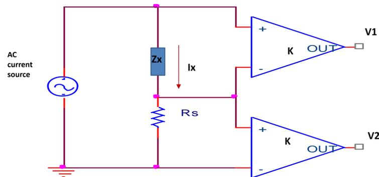
Fig. 2. The circuit diagram for the RLC meter (RLC Digibridge®) [2].
