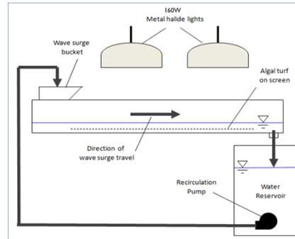
Figure 3: Schematic of lab-scale recirculating ATS used in this experiment
