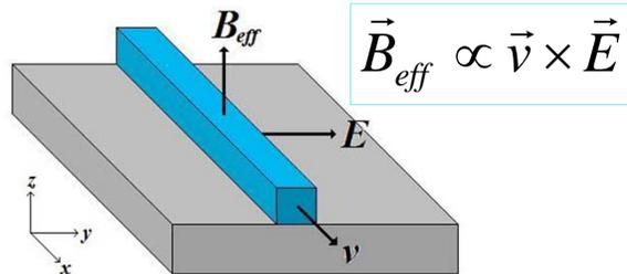
This field is added vectorially to any external applied magnetic field. The total field then interacts with the magnetic moment of the electron, causing Zeeman Splitting:
